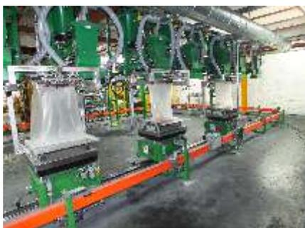
Automatic systems for bucket, container and bulk IBC can also be supplied although the latter would normally be located upon a linear track. Due to the unique philosophy of the Smart cart it is possible to incorporate additional feed stations and track extensions at a later date if expansion should be required.
