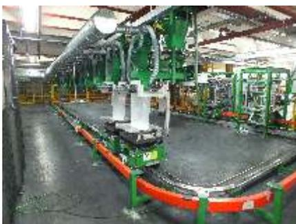
This system can also reduce / eliminate costly downtime due to weigher malfunctions as each weigh carriage can be simply removed from the track for maintenance or repairs. The remaining carriages will then continue the weighing operations or an additional spare carriage can be added to maintain the same throughput.
