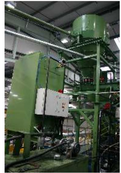
Material is transferred to the receiving vessel which is fitted with a reverse jet filtration system which separated the transferring air from the material via a series of filter cartridges. The cartridges are automatically cleaned between batches using reverse air jets.
