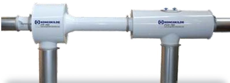
The venturi system works by creating a constriction within the pipe (classically a hourglass shape) that varies the flow characteristics of the gas travelling through the tube. As the velocity in the throat is increased a consequential loss in pressure occurs. This drop in pressure therefore creates a vacuum effect which can be used to draw material into the conveying pipeline. On the downstream side of the venturi unit the material is conveyed using the positive pressure air flow.
