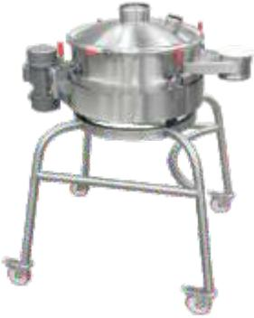
Circular vibratory screens are designed for all product applications from food sectors to aggregates, in either wet or dry applications. Screening assembly is mounted on reactive springs and can be supplied in a multi-deck system giving up to four fraction separation. Each deck is secured with quick release clamps allowing rapid cleaning and mesh changing when required.
