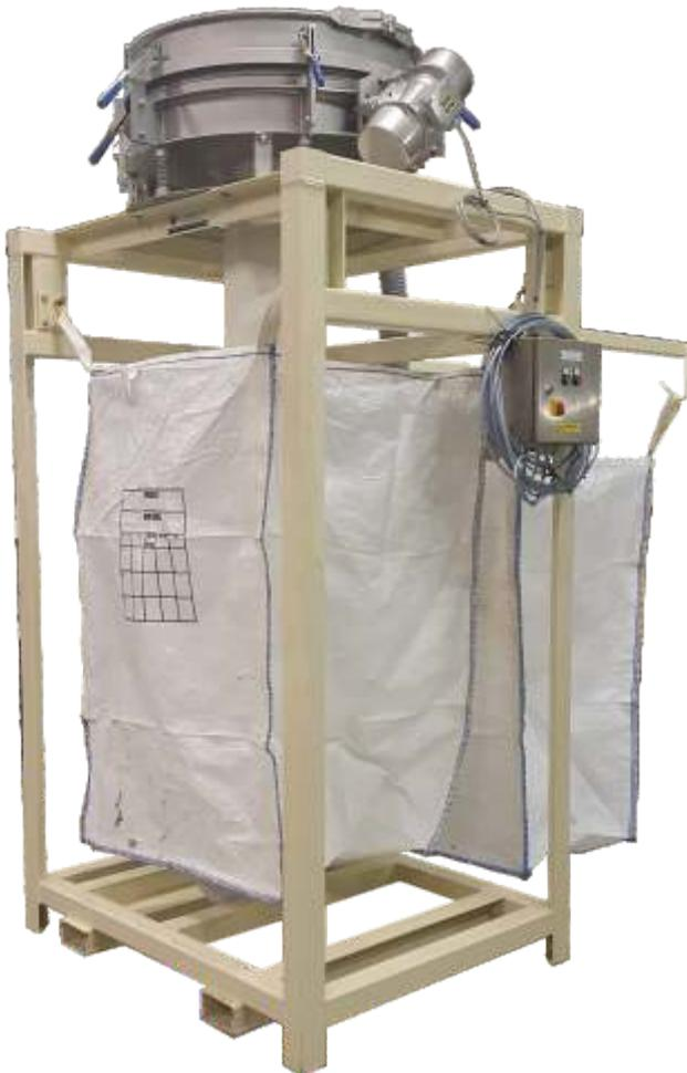
Both linear and circular sieves can be custom designed together with bespoke frameworks to allow incorporation within your specific plant process. From direct bulk bag filling solutions to custom separation systems we can develop a system concept to fulfil your specific separation and sieving requirements.
