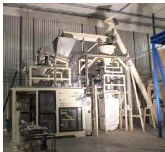
Material is fed from the holding hopper via an inclined transfer screw to a twin outlet dosing screw which discharges to either the bulk bag or the sack filling line.
