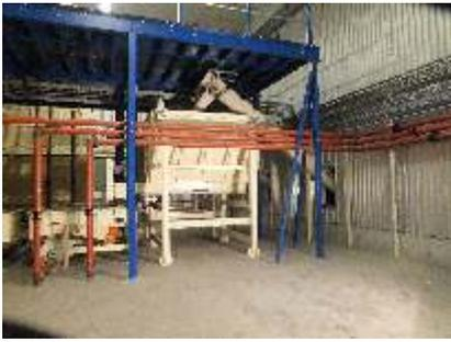
The two external bulk silos each feed directly into two dedicated batch weighers located just inside the building. This is done via screw feeders with automatic shut-off valves passing through the building wall.
