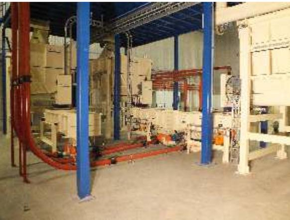
The three vibratory screens are situated at the in-feed point of the pneumatic conveying system and remove any oversize particles. Material is then dispensed into the conveying line via blow through rotary valves.
