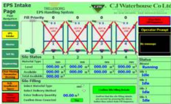
The intake panel is located adjacent to the EP unloading area and incorporates a HMI unit providing specific information relating to the EP intake system. This display provides system information, controls, alarm monitoring, configuration and allows the operator to set the delivery type, intake material, silo destination and conveying parameters.
