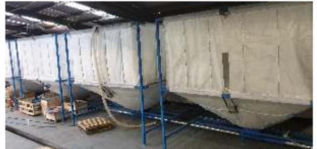
The storage facilities comprise of Polypropolene fabric hoppers suspended from mild steel frameworks and incorporate viewing windows and filtration membrane on the upper face for removal of conveying air. Each silo is fitted with ultra sonic level detection systems and a pneumatically operated discharge slide valve.
