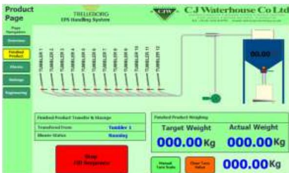
The out-loading panel is located adjacent to the finished product weighing system and incorporates a remote I/O module providing automated control of the finished product conveying, storage and weighing system. This panel also incorporates a HMI display providing operator information for the tote bin filling and weighing system.
