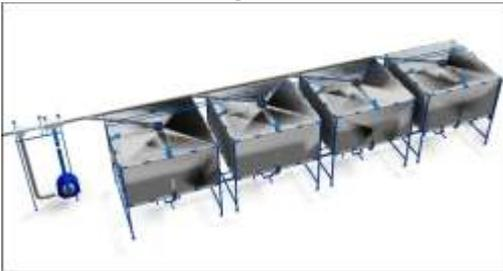
The bulk intake system accepts EPS deliveries in either tote bins or bulk tanker format and conveys it to four 65M3 fabric silos via a venturi conveying system providing negative pressure extraction at the infeed point and positive pressure conveying to the receiving silos. The materials are transferred through a single conveying line to the four silos via three diverter valves.
